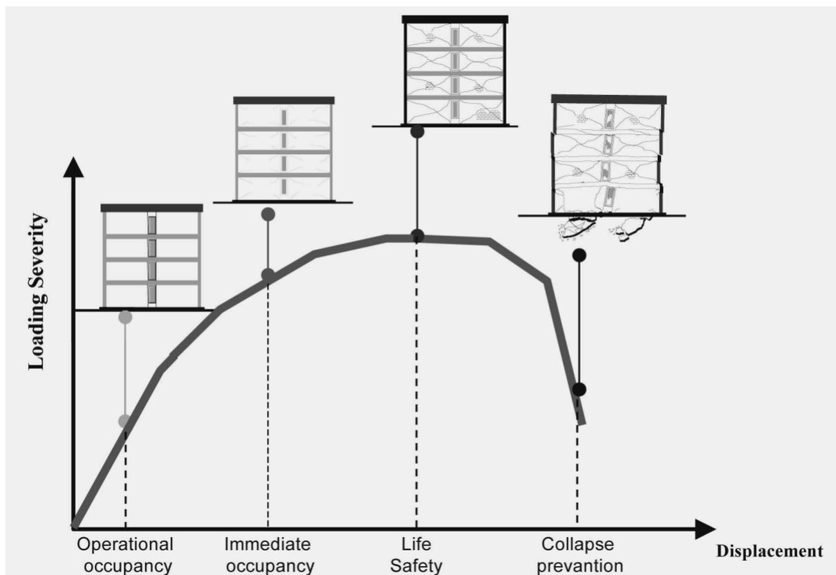
Figure A-XI. 1: *Illustration of Building Performance Levels*
