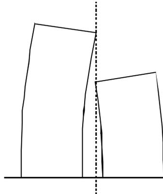
**Figure A IV-4:** *Sufficient gap between two buildings prevents pounding*
